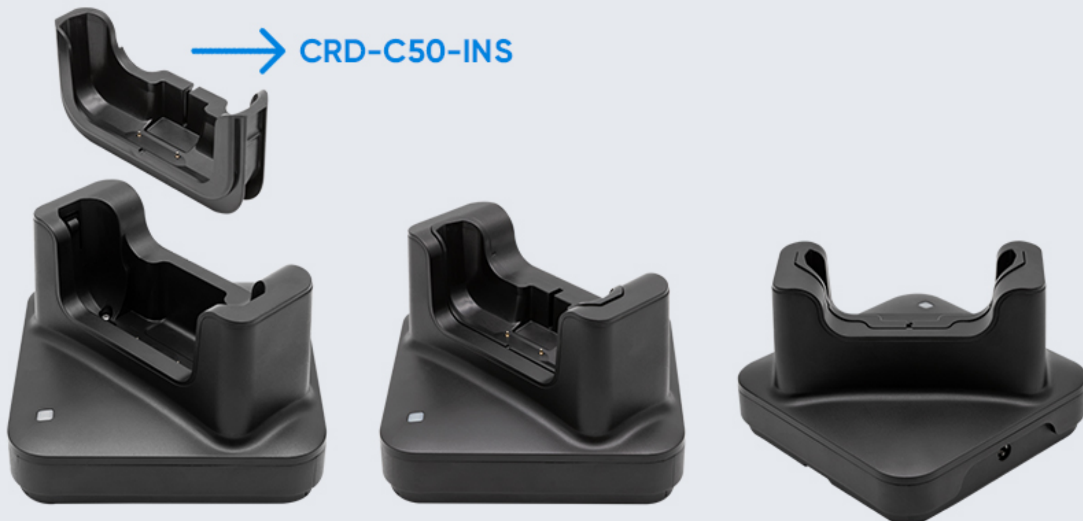
CRD-C50-DP Charging Cradle for device, include the cradle cup(CRD-C50-INS),support device with UHF pistol grip or only device, use with DCPWR-12V2A-XX adapter. The cradle cup has an insert that must be removed prior to inserting the MC50 with UHF pistol.
